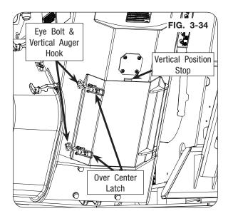
8. Rehook eye bolt to vertical auger and clasp the over center latch.
