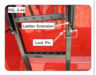
3. With hands back on ladder handles, push ladder towards hopper bin and lift ladder extension to unseat ladder extension rod from the cradle. (FIG. 3-45)
