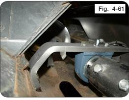
24. Extend a string tightly from front to rear to check horizontal auger alignment. Measure the string to the auger tube either in front or behind the hanger bearing. If this dimension is 1/8" greater than the measurement taken in the front and rear, shims (8GA - 286419B or 12GA - 286424B) are required on top of the center hanger bearing. Ideally the center measurement should be equal to or 1/8" lower than the measurements on the ends of the augers. (Figure 4-62)
