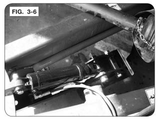
Use hydraulic jack to support an empty grain cart, never a loaded grain cart. Always have a loaded grain cart hooked to tractor.
