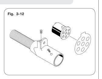
If equipped, check the tractor and cart electric tarp connection. Refer to electric roll tarp manual (26487) for details.
